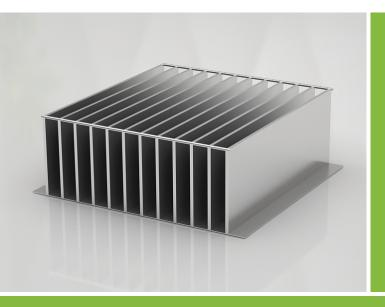
The corrugated wall panel / fin walls are directly welded to the transformer tank. Besides the obvious advantage of reduction on the overall dimension of the transformers, the thermo power wastage is lower and the flow of oil does not become sluggish hence the efficiency of the radiators is better. This in the long term improves the usable life of the transformer and maintenance cost is lowered.
